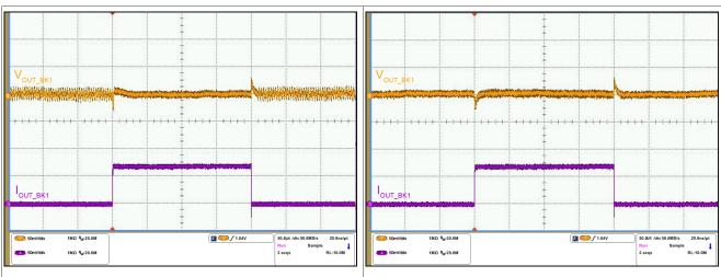
Figure 14. Buck1 (1.1V) load transient response 100 mA to 750 mA
