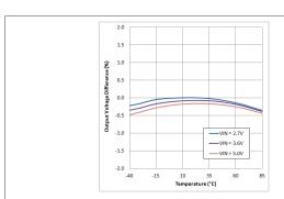
Figure 41. Buck1 Output Voltage Error vs Temperature
