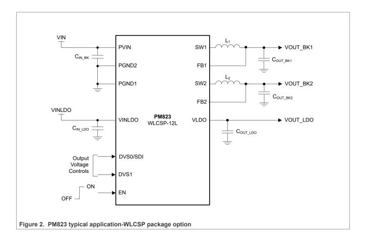
Dual Synchronous 1.5A/1.5A Step-down Buck Regulators with 525 mA LDO
