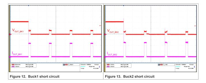
Dual Synchronous 1.5A/1.5A Step-down Buck Regulators with 525 mA LDO
