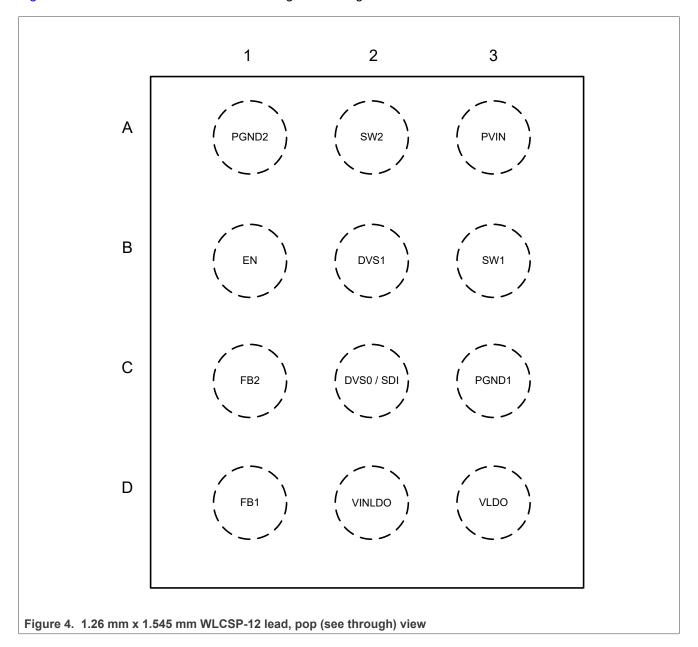
Dual Synchronous 1.5A/1.5A Step-down Buck Regulators with 525 mA LDO
