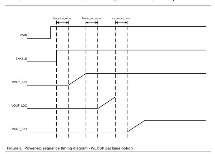
Dual Synchronous 1.5A/1.5A Step-down Buck Regulators with 525 mA LDO
