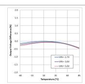
Figure 42. Buck2 Output Voltage Error vs Temperature
