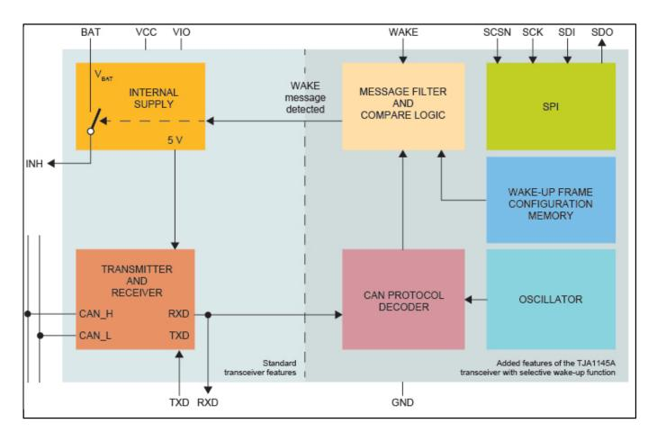
View additional information for High Speed CAN Transceiver with Partial Networking, CAN FD Data Rates up to 5 Mbit/s.
