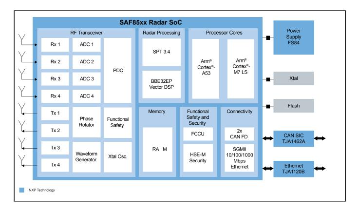
View additional information for High Performance 77GHz RFCMOS Automotive Radar One-Chip SoC.
