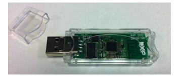
Figure 28: JN5169 USB Dongle
