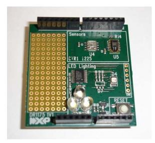
Figure 23: Lighting/Sensor Expansion Board
