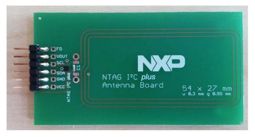
Figure 31: NTAG I<sup>2</sup>C plus Antenna Board
