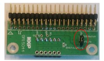
Figure 33: J16 Jumper on OM15044 Adaptor
