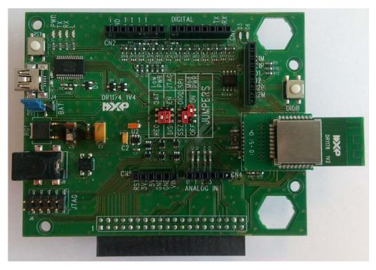
Figure 16: Carrier Board (with a JN516x Module)
