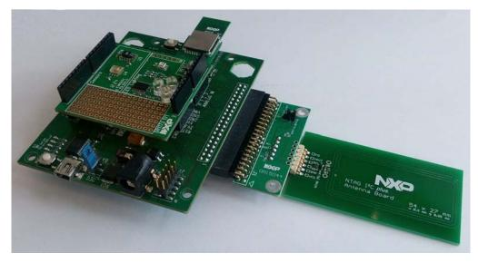
Figure 32: Fully Assembled Board with NFC Tag
