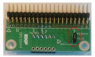
Figure 13: J16 Jumper on OM15044 Adaptor
