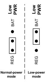
Figure 19: Lower-Power Mode Selection (using Low PWR Jumper)
