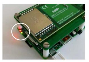
The IoT Gateway is then ready. When in this state, the green LED on the NFC Controller board flashes.
