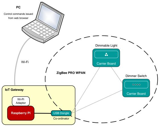
Figure 11: ZigBee Smart Home Demonstration System
