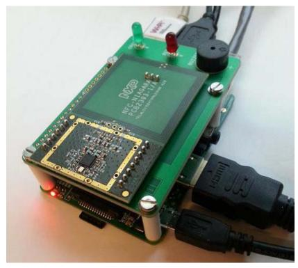
Figure 30: NFC Controller Assembly on Raspberry Pi Board
