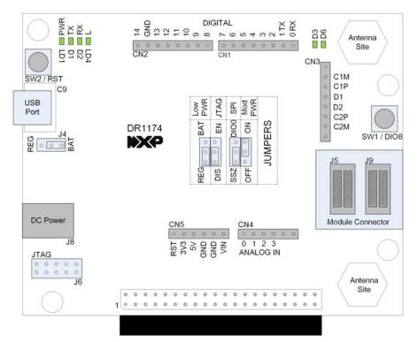
Figure 15: Carrier Board Layout
