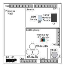
Figure 22: Lighting/Sensor Expansion Board Layout
