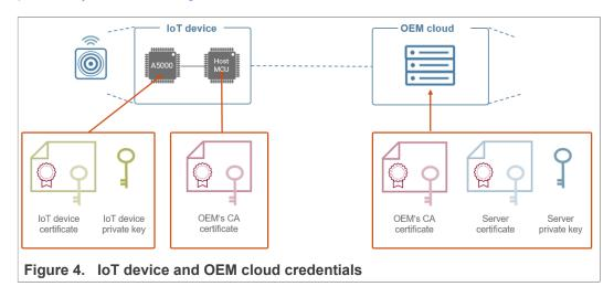
Security ICs chips like A5000 are capable of internally protecting private keys in IoT devices. The CA certificate is typically stored outside the A5000. Section 4 outlines the A5000 trust provisioning models available.
