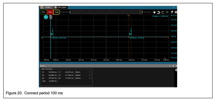
Following is an example of a sniffer capture of a Connect event.
