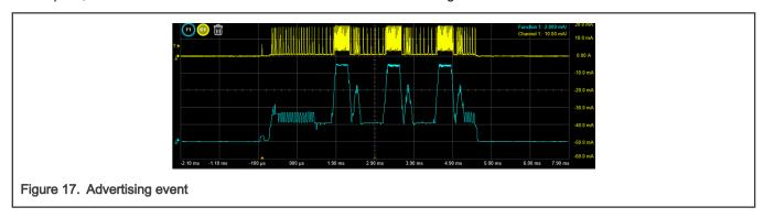
The power profile is analyzed and the energy consumption can be measured at 6.288nAh under 3.0 V. The total event duration is 5.64 ms.
