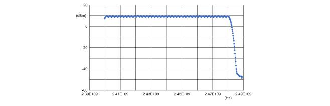
Figure 8. TX power for 2 MB/s
