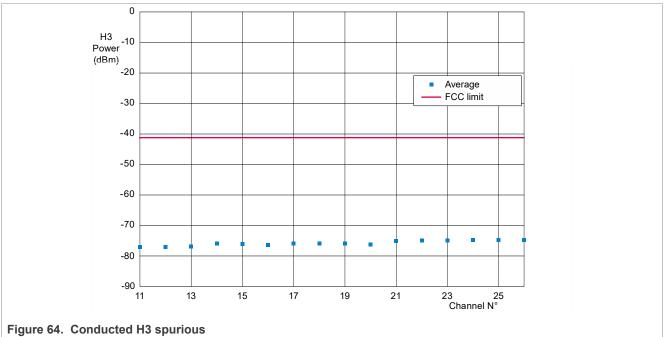
• Maximum power is on channels 21 to 26: -75 dBm
