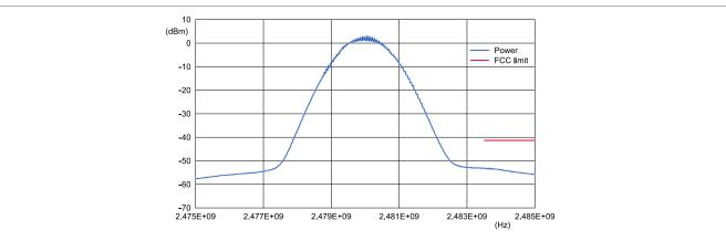
Figure 25. Upper band edge for 1 MB/s, channel 39
