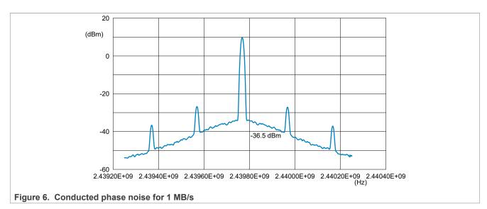
• Marker value (delta) = -46.1 dBm / 100 kHz = -86.1 dBc/Hz
