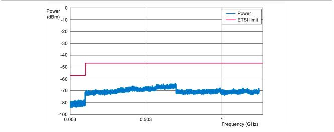
Figure 36. Conducted RX spurious 30 MHz - 12.5 GHz
