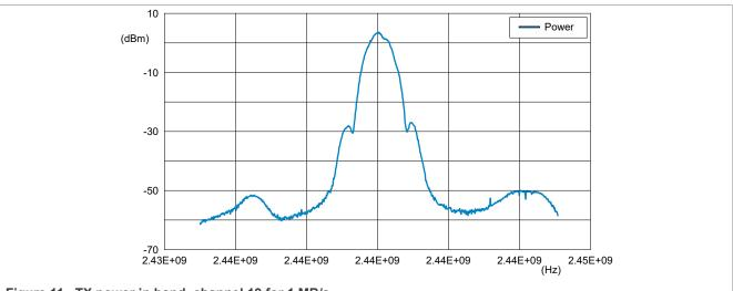
Figure 11. TX power in band, channel 19 for 1 MB/s
