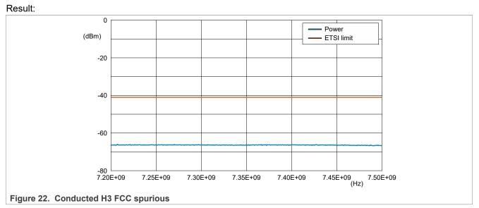
· Power is -66 dBm below the noise floor of this measurement.
