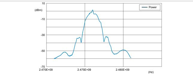
Figure 14. TX power in band, channel 37 for 2 MB/s
