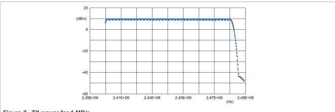
Figure 7. TX power for 1 MB/s
