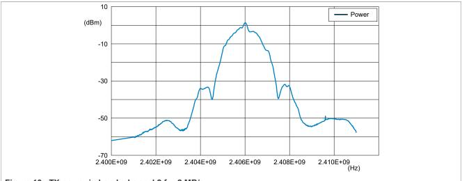
Figure 10. TX power in band, channel 2 for 2 MB/s
