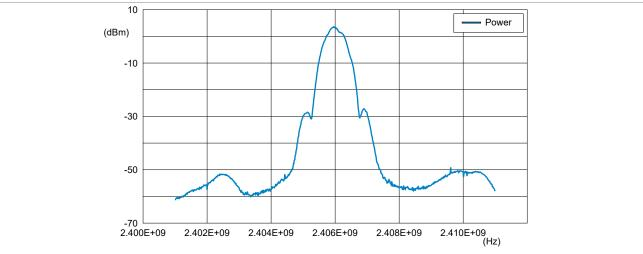
Figure 9. TX power in band, channel 2 for 1 MB/s
