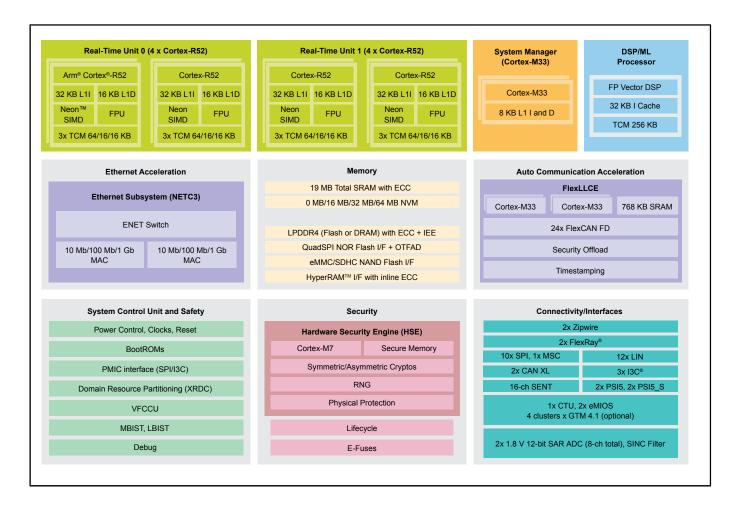
S32Z and S32E Real-Time Processors Software Block Diagram Block Diagram
