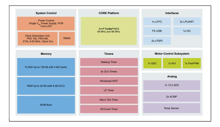
View additional information for MCX A14x/15x MCUs with Arm® Cortex® M33, Scalable Device Options, Low Power and Intelligent Peripherals.
