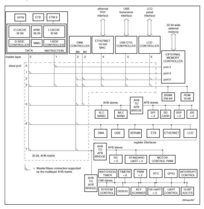
View additional information for Arm926EJ-S™ with 256 KB SRAM, USB High-Speed OTG, SD/MMC, Nand Flash Controller, Ethernet, LCD Controller.
