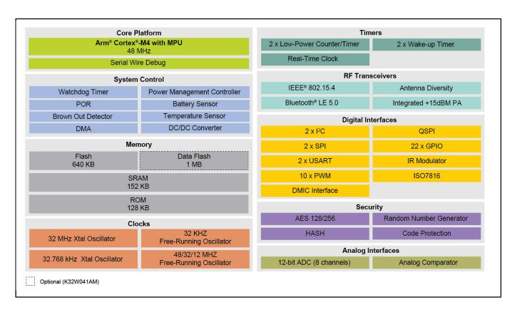
View additional information for K32W041AM/A: High Performance, Secure and Low-Power MCU for Zigbee®, Thread™ and Bluetooth® LE 5.0 with High Tx Power Option.
