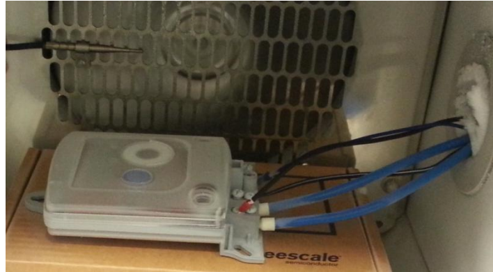
Figure 8-2. Power meter inside a heat chamber – temperature controlled to -40 °C
